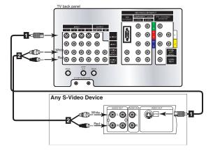
Figure 2. Connecting an S-Video Device.
